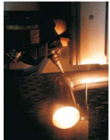
Above: The 3D laser cutter offers a diverse range of complex jobs including counter sinking of holes and slots on plates and pipes, bevel edging of blades, mitring of plates for weld preparation and creating perfect monolithic joint points on RHS and tubing. Photos: Schulz
