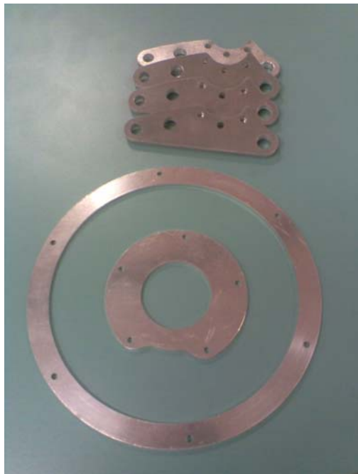
Above: Laser cut parts of the bellcrank plates (TOP) and bearing carriers (BOTTOM) for the ts_07 car.
