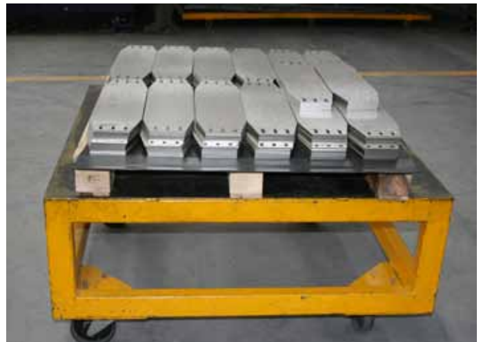
Using part trolleys has reduced trip and cutting safety hazards, and cut reliance on forklift use.
